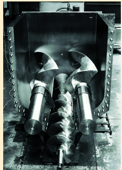
The two powerful Sigma blades of the Kneader Extruder fold and compress dense material at lower temperatures – an important advantage for mixing heat-sensitive materials. The extrusion screw increases shear during mixing, then turns in reverse to accelerate discharge.
